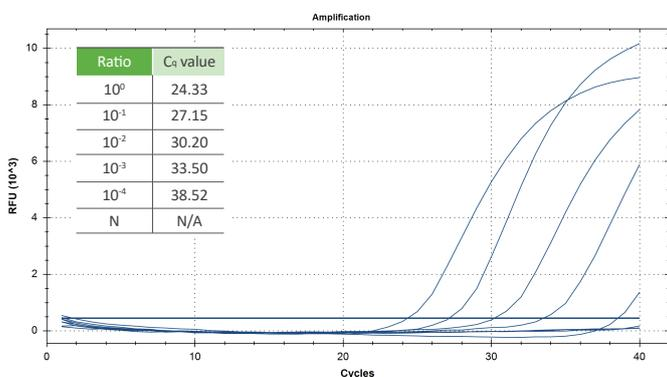
**Figure 2.** Analysis of extraction sensitivity on serial dilutions of *Mycoplasma gallisepticum* (MG). The DNA templates were extracted from a 10-fold serial dilution of *Mycoplasma gallisepticum* (MG) using Exgene™ Viral DNA/RNA. All eluates were analyzed with a TaqMan-based real-time PCR assay using CFX-96.
